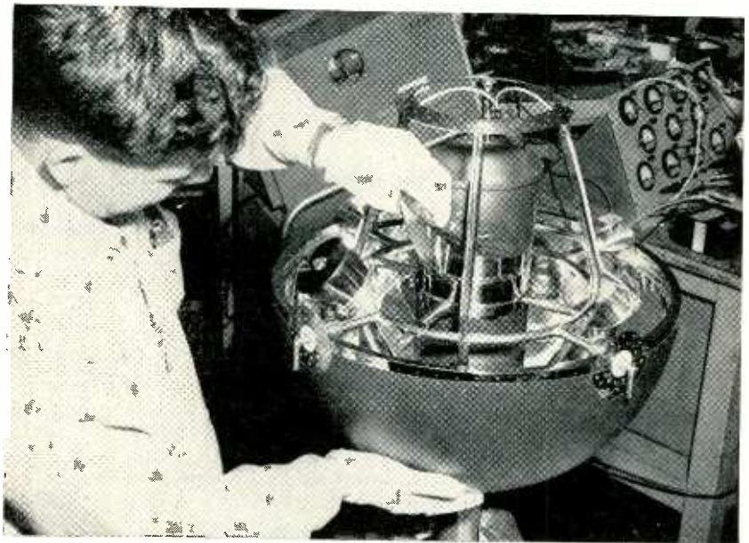
Interior of satellite is plated with about 2-oz of pure gold to maintain even temperature during flight. Photoelectric pickups are mounted on opposite sides of housing
