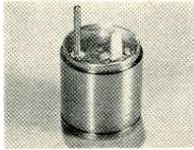
Ceramic window is brazed into a partition which, in turn, is brazed into tube envelope. Pin is locating device
